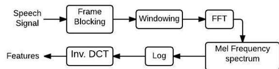
Fig. 2. Block diagram of extracting the MFCC features.
