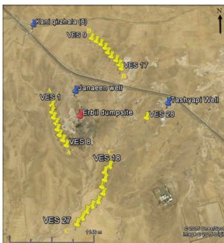
Fig. 5 Map showing the vertical electrical sounding points and calibration wells at the study area
