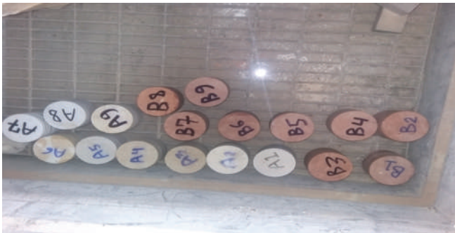
Fig. 2. Eighteen Different Core Samples Collection from Limestone and Claystone of Fatha Formation for Laboratory Tests.
