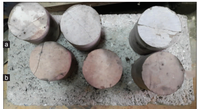
Fig. 6. Cracks in Limestone (a) and Claystone (b) Generated due to High Temperature.
