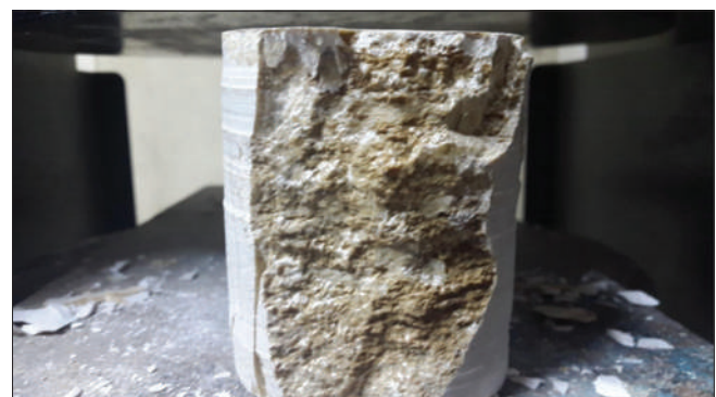
Fig. 7. Limestone Core Sample show Deformation due to Exposure to 650°C.
