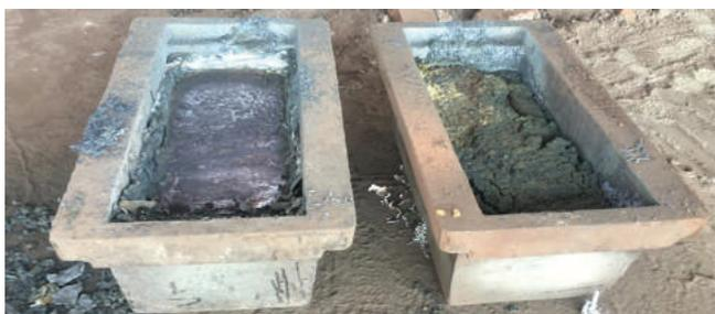
Fig. 7. Two metal pouring cases, the right one with matt and the other without.
