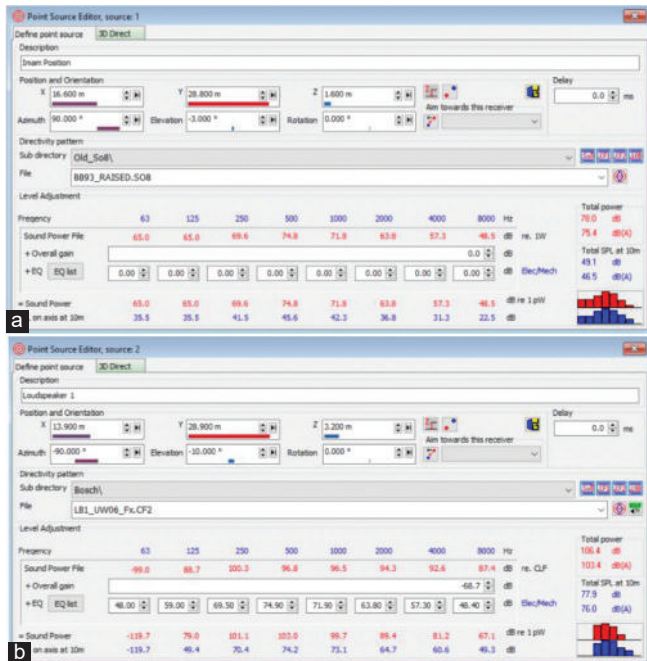
Fig. 4. Point source editor setup in ODEON, (a) imam source, and (b) loudspeaker source.
